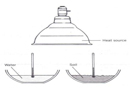
each container. Temperature readings were recorded each minutes during both the heating and cooling periods. The results of the investigation are contained in the Data Table on the next page.
